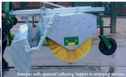
Sweeper with optional collecting hopper in emptying position
