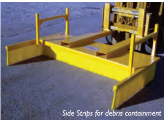
Side Strips for debris containment
