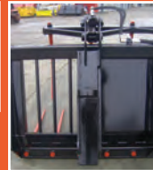
Quick Hitch Brackets in line with Ram Pivot Points
